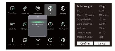
Press the UP/DOWN button to adjust the values of the parameters.
